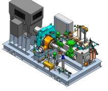
Energent's EULER TURBINE technology was applied to a KALINA CYCLE geothermal power plant in Bruchsal, Germany. The RADIAL OUTFLOW turbine rotates at 28,000 rpm, allowing the use of a single stage gearbox as opposed to a two-stage gearbox which would be required by a radial inflow turbine. Its rugged, TITANIUM ROTOR provides corrosion and moisture resistance to operate with the saturated vapor supplied by the KALINA CYCLE.
